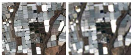
Figura 5. Izquierda: Ortho Imagen MS (1.6 m) WV2, 30 Sept. 2013. Derecha: Ortho Imagen pansharpened (15 m) Landsat 8, 12 Sept. 2013.
