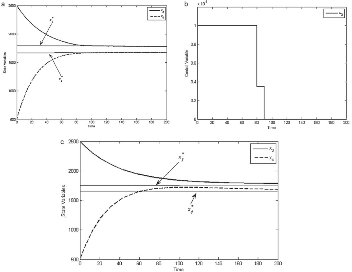
Fig. 3. (a) Solution of control system (3.9) for  $T=200$ , with initial value  $x^{02} := (2500, 500)$ , (b) control function of system (3.9) for  $T=200$ , (c) solution of the uncontrolled system (3.6) for  $T=200$ , with initial value  $x^{02} := (2500, 500)$ .
