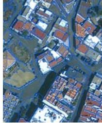
Multiresolution segmentation using eCognition 8.0. 4 pan-sharpened bands plus PAN band. Scale = 50, Shape = 0.3 and Compactness = 0.7
