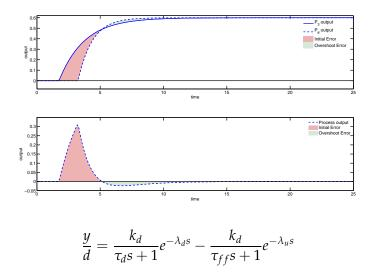
From the previous analysis, it can be concluded that in order to totally remove the overshoot for the disturbance rejection problem by using a lead-lag filter, the settling times of both transfer functions must be the same:
