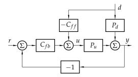
$$Y = \frac{P_d - C_{ff} P_u}{1 + C_{fb} P_u} D, \quad C_{ff} = \frac{P_d}{P_u}$$
