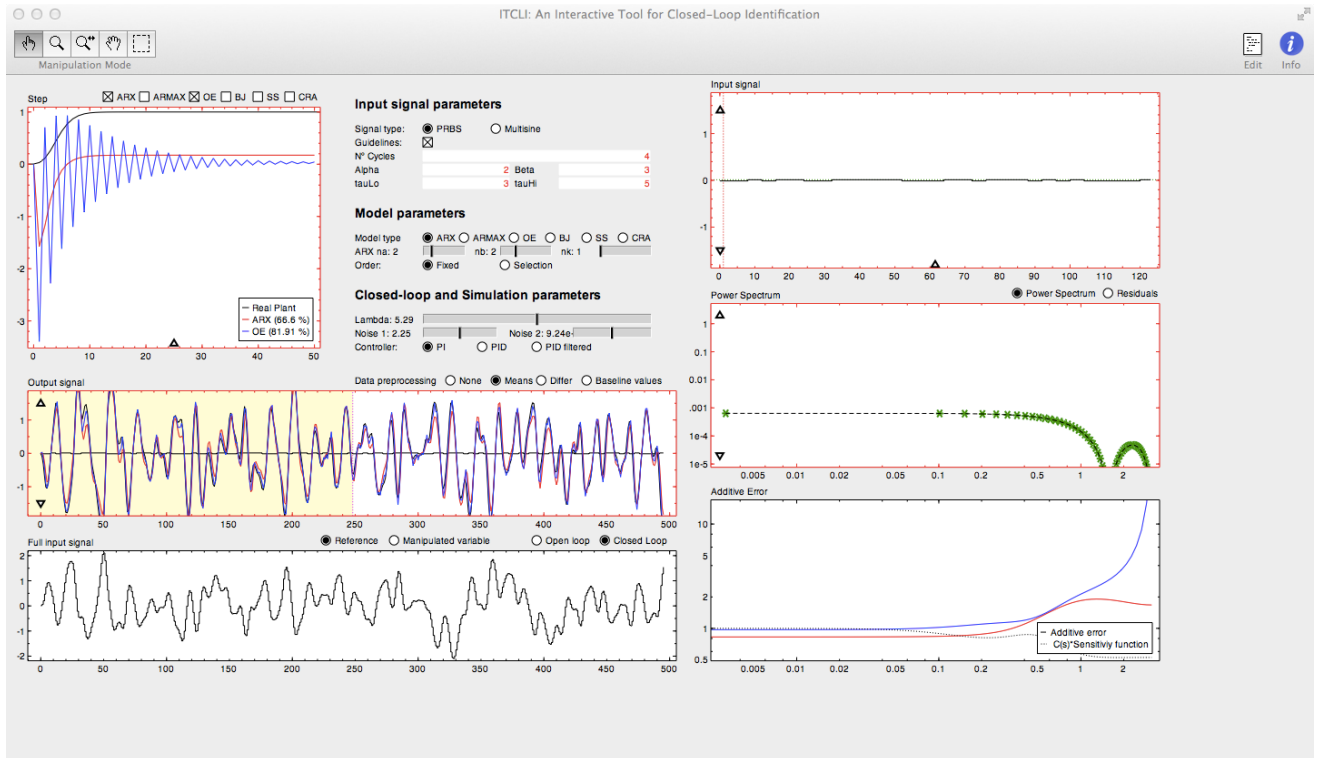
Fig. 4. Results for the third illustrative example explained in Section 5. If only excitation from disturbances is considered, it is possible in closed-loop identification to fit to data “perfectly” with highly erroneous models. This motivates the need for a sensibly designed external input signal.
