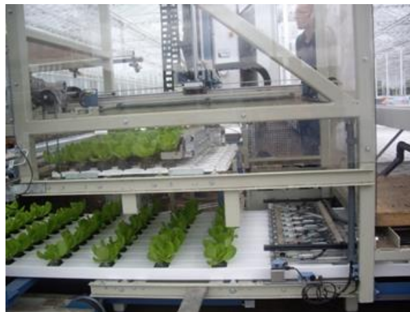
Figure 9-11. Automatic transplantation of lettuce from plastic crates to the gutters (Source: Isabel Vandevelde)
