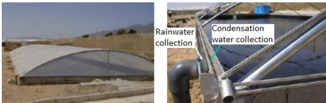
Figure 2-39. Picture of closed greenhouse used as passive solar desalination system
