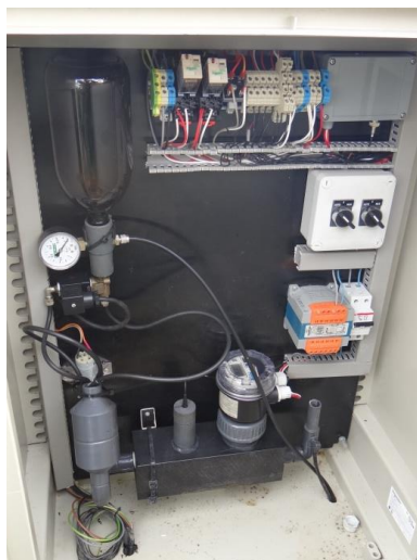
Figure 11-10. Equipment for automatic suction and EC and pH measurement of soil solution produced by Himarcán, Almería, Spain
