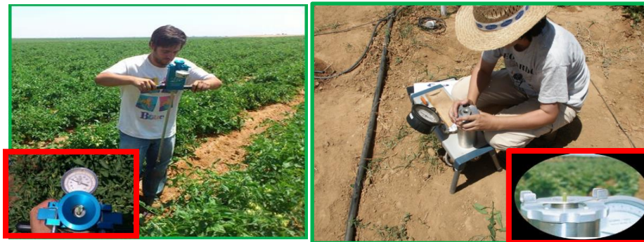
Figure 10-25 Measure water potential with pump-up system in processing tomato crop (a) and console chamber system with tank (b) (Source: CICYTEX)
