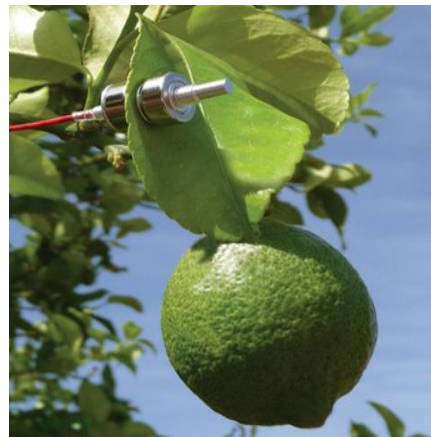
Figure 10-22. Yara water sensor
