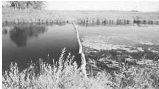
Figure 5-7. A pond divided in two to demonstrate the efficacy of the addition of lime in order to control algal bloom. The picture shows the situation after the treatment. The left side shows the treated water volume, the right side shows the untreated water
