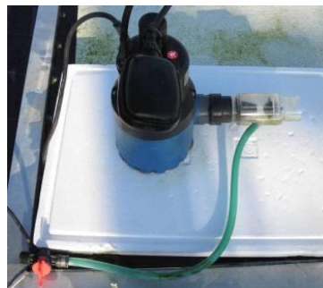
Figure 6-23. Submersible pump with an extension for aeration based on the Venturi principle
