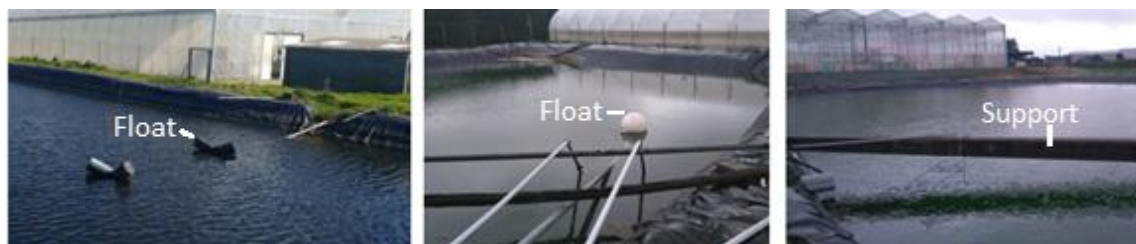
Figure 2-45. Examples of different constructions of floating pumps. Left and middle: pumps attached to floats; Right: floating pump attached to a fixed structure, in this case, a pole (Source: CATE)
