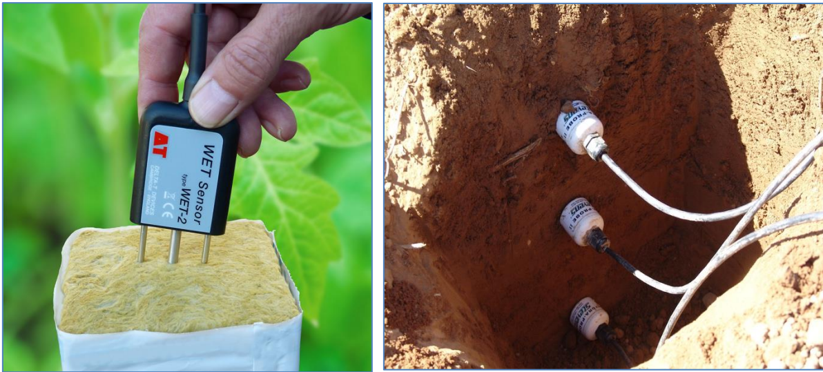
Figure 10-27. WET sensor used to take measurements on rockwool and soil in open air ( https://www.deltat.co.uk )
