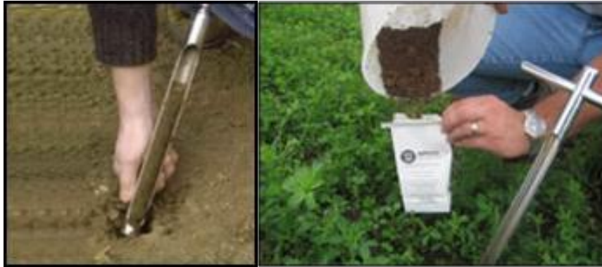
Figure 11-5. Taking a soil sample with an Auger and collecting the sample ( http://cri.crinet.com/news2536/PlanNowForSpringSoilSampling )
