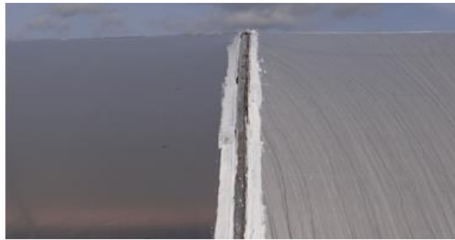
Figure 2-38. Behaviour respect to condensation of different plastic types: left, anti-drip plastic with film condensation; right, conventional plastic with dropwise condensation
