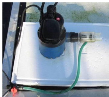
Figure 6-24. Submersible pump with an extension for aeration based on the Venturi principle
