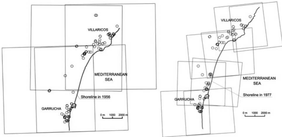
FIG. 2. Configuration scheme for photography, ground points and shoreline in the two archival datasets tested: 1956 (left) and 1977 (right). Note that the coastline position limits the collection of an optimal distribution of GCPs.
