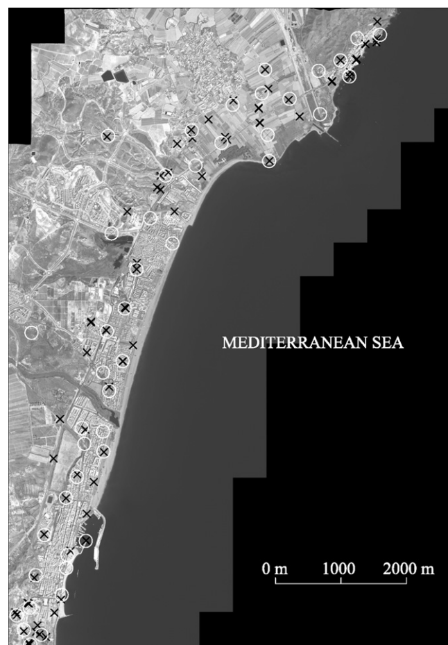
Fig. 2. Distribution of 75 ICPs (black crosses) and 44 GCPs (white circles) overlaid on a GeoEye-1 panchromatic orthorectified image.
