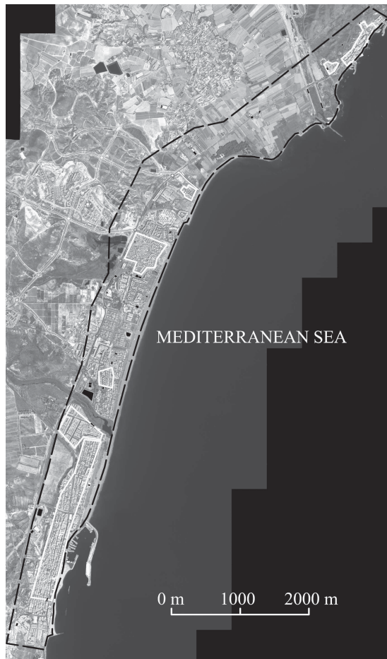
Fig. 2. Different areas for assessing the quality of DSMs overlaid on a GEI orthoimage. Urban areas in white, unchanged areas in solid black and the whole working area in black dashed line.
