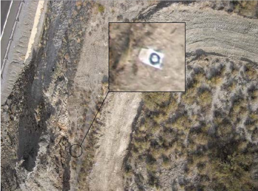
FIG. 3. Target points detail from one of the photogrammetric project image.
