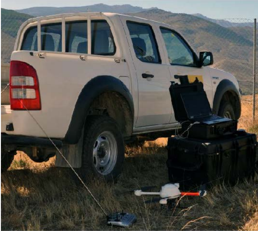
FIG. 2. UAV Microdrones model md4-200, base station and hand held remote control transmitter. Both the flight routes and flight controls were planned and programmed, respectively, using the md-Cockpit Standard Edition V2.8.0.6 software package, which is compatible with the Microdrones UAV.
