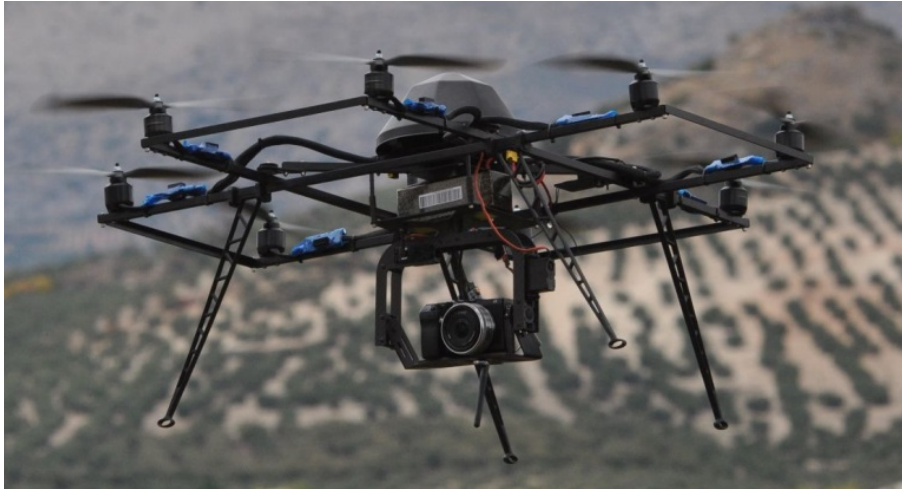
Figure 2. The UAV oktokopter used in this work as photogrammetric platform.
