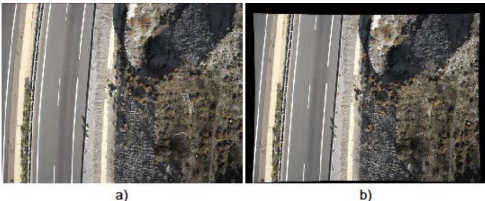
FIG. 6. (a) One of the original images taken in the flight (b) the same image after distortion error correction.
