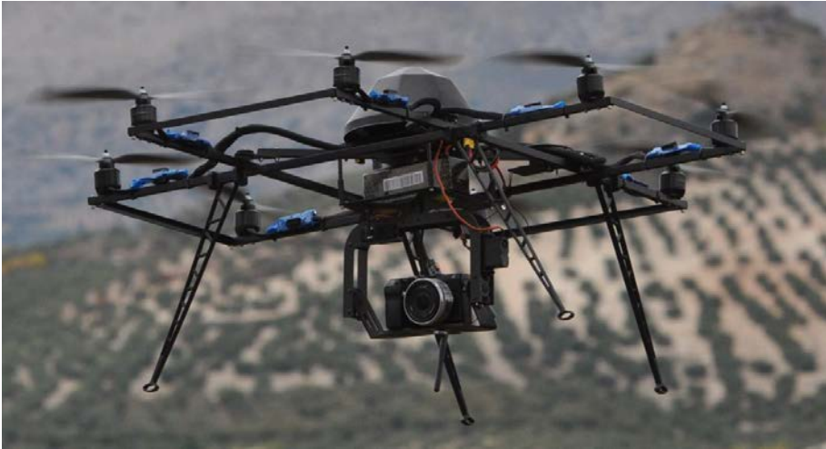
Figure 3. UAV oktokopter used as a photogrammetric platform.
