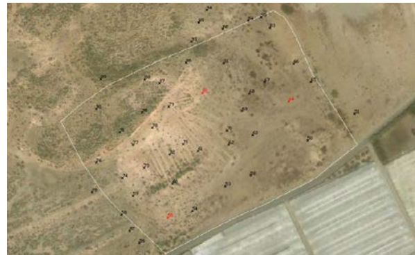
Fig. 19 Ground control points (red) and check points (black) for the photogrammetric block orientation and accuracy control, respectively.
