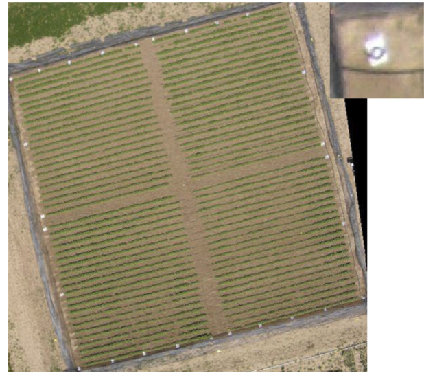
Fig. 4 – Field experiment RGB image with targets for elemental plot identification and georeferencing. In the upper right corner, a detailed enlargement of a target image is shown.
