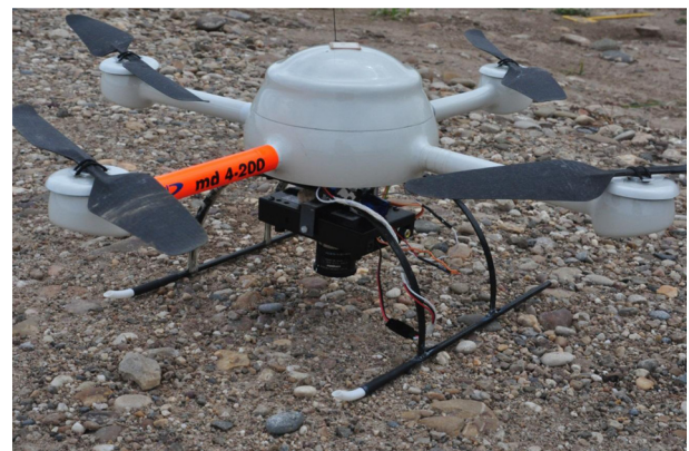
Fig. 2 – The Microdrones MD4-200 UAV with Tetracam ADC Lite that was used for image acquisition.
